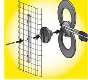
Attach the two cross bars (6) (with mounting hardware) to the rear of the reflector (1) by removing the back clamp, threading screw and clamp back on and screwing on wing nut (5). Note: Screws should be poking through the back of the reflector.
